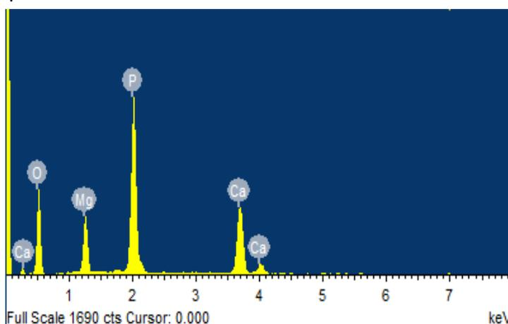
Figure 6. EDS spectrum of  $\text{DCP}_{\text{recovery}}$  sample.
