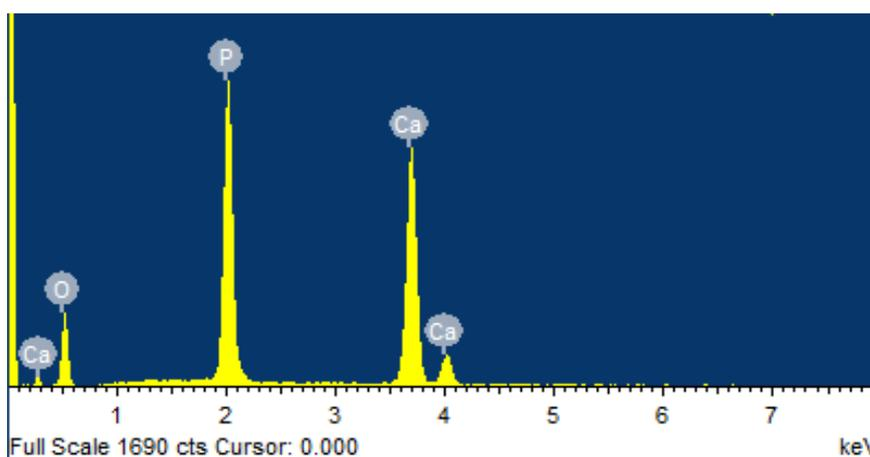
Figure 3. EDS spectrum of M2.5 sample.
