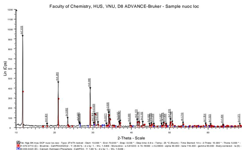
Figure 4. XRD diagram of  $\text{DCP}_{\text{recovery}}$  sample.
