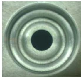
Figure 1. Hot-forged die geometry used in this research.
