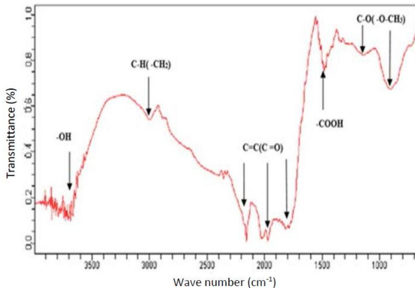
Figure 2. FTIR analysis of biochar CFH 350.
