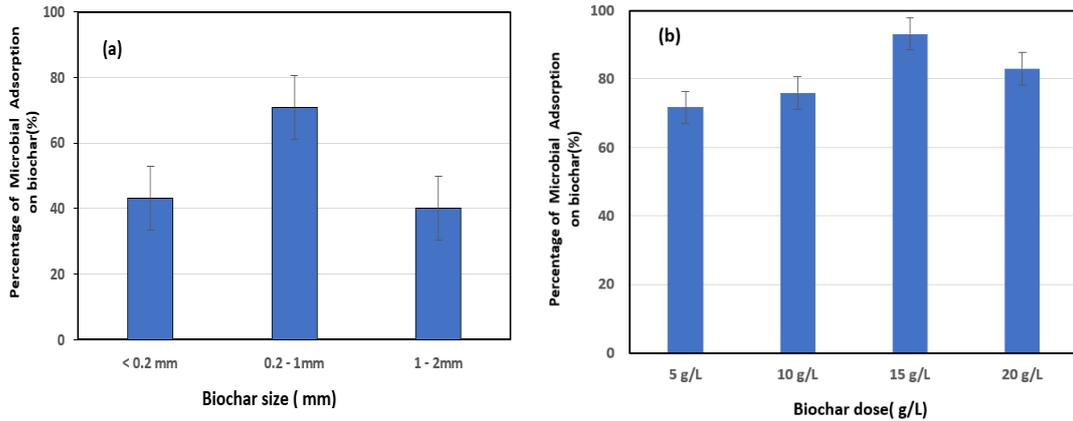
Figure 4. Effect of biochar size (a) and biochar dose (b) on microbial adsorption.
