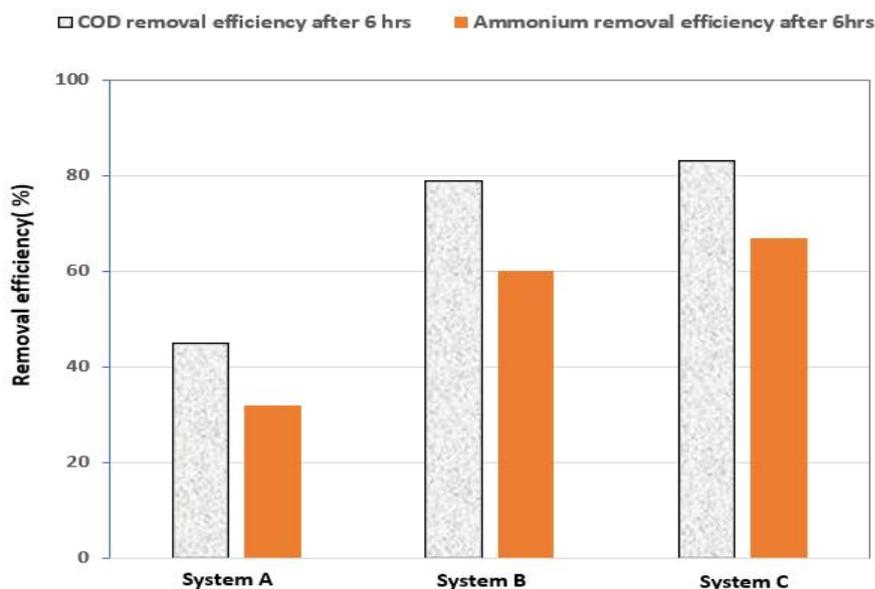
Figure 6. Removal efficiency of COD and ammonium in different system.
