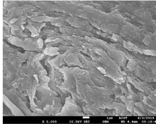
Figure 1. SEM of Biochar CFH 350.
