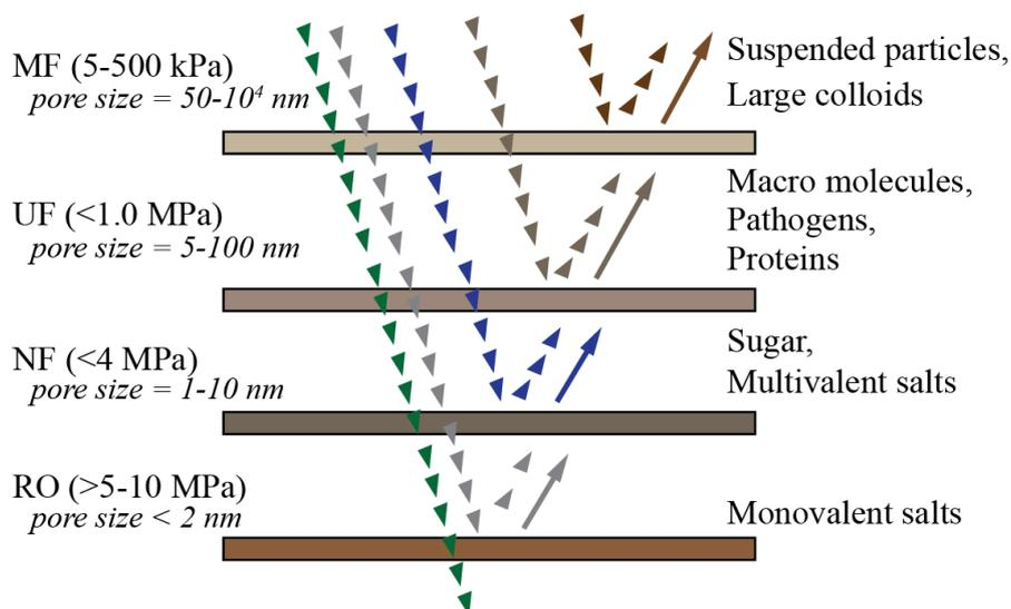
Figure 1: The ranges of pore sizes, applied pressure, and applications of pressure-driven membrane processes
