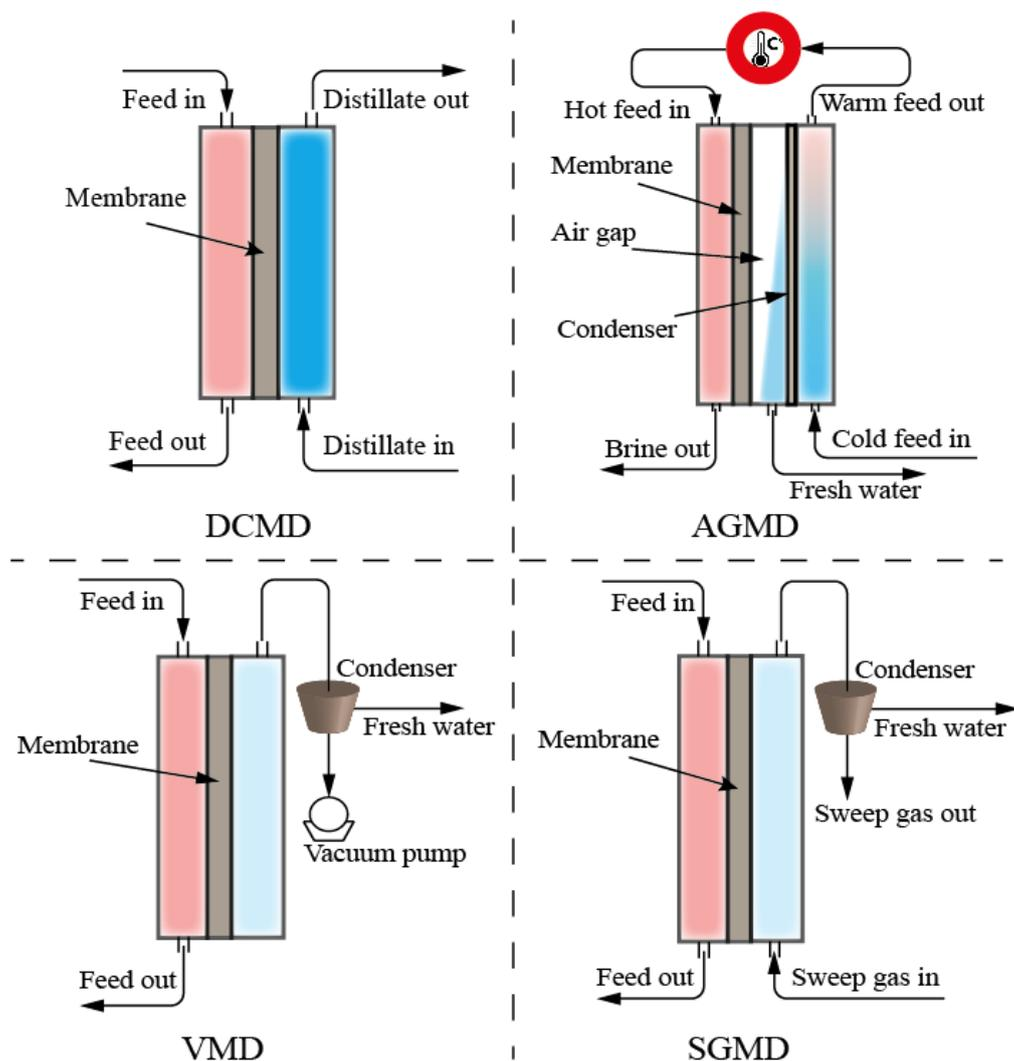
Figure 5: Four basic configurations of MD
