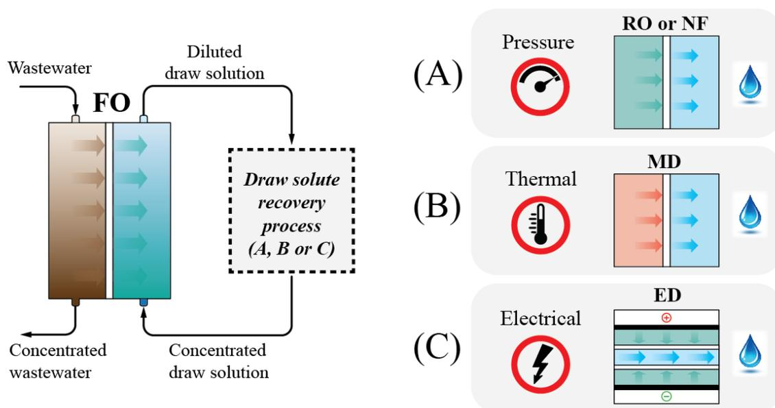
Figure 4: A schematic diagram of an FO process with various draw solution regeneration methods
