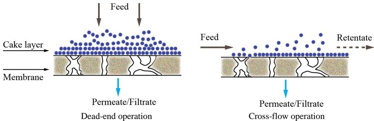
Figure 2: Dead-end and cross-flow operation modes during the MF/UF separation process
