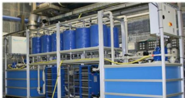
Figure 6: Photographs of pilot MD membrane modules and system
