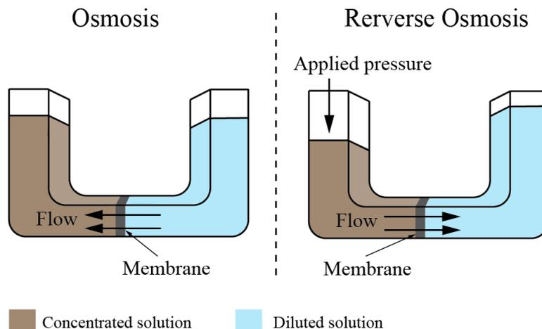
Figure 3: Principles of osmosis and reverse osmosis process
