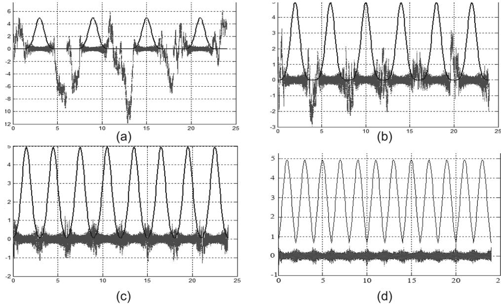
**Fig. 6.** Stability process of particle in optical tweezer pumped by series of laser pulses with different repetition period. (a):  $T = 6\tau$ ,  $n = 4$ ; (b):  $T = 4\tau$ ,  $n = 6$ ; (c):  $T = 3\tau$ ,  $n = 8$ ; (d):  $T = 2\tau$ ,  $n = 12$ . **Note:** Vertical unit [nm]; Horizontal unit [ $\tau$ ].
