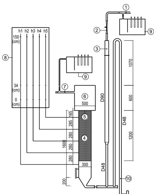
*Figure 1.* Pilot model of hydraulic automatic floating media filter for advanced wastewater treatment. (1) influent of wastewater from secondary biological treatment; (2) ejector; (3) hydraulic pressure stabilizer; (4) polystyrene filter media bed; (5) grit; (6) backwashing tank; (7) effluent of treated wastewater; (8) Piezometer Panel; (9) Online control facility ( $q$ , COD, SS,  $\text{NH}_4^+$ ); (10) Backwashing siphon.
