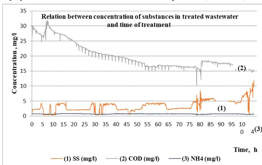
Figure 2. Relationship between SS, COD and  $\text{NH}_4^+$  concentration in effluent treated wastewater and time of filtration.
