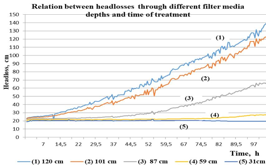
Figure 3. Headloss development during filter operation cycle (filtration velocity  $v = 4$  m/h).
