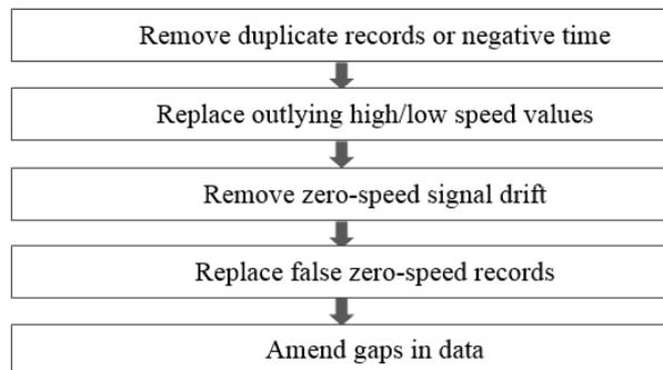
Figure 3. Flowchart of GPS data filter.
