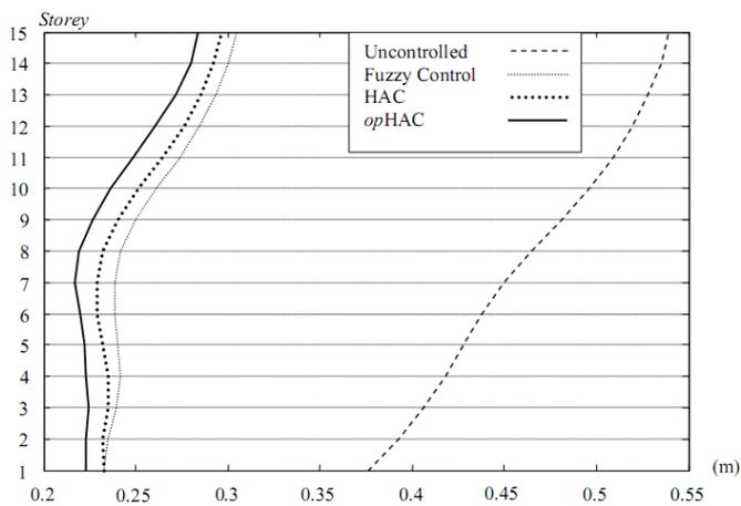
Figure 14. The maximum storey drift – Kobe earthquake
