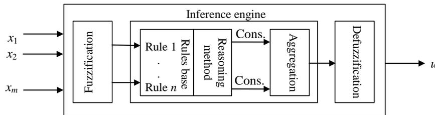
Figure 1. A schematic view of the fuzzy controller
