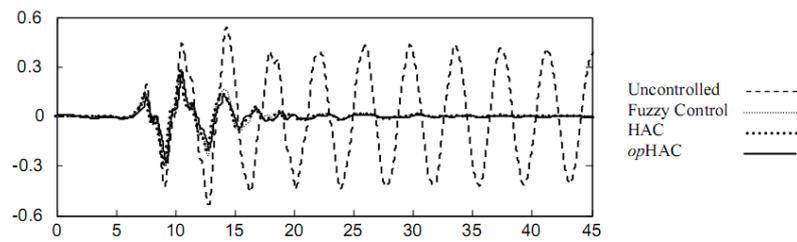
Figure 15. Displacements  $x_{15}$  versus time - Kobe earthquake
