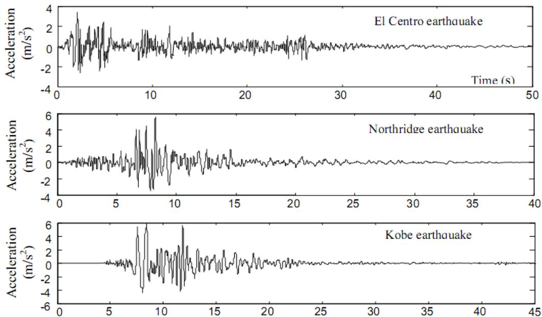
Figure 5. The ground acceleration  $\ddot{x}_0$  ( $m/s^2$ )
