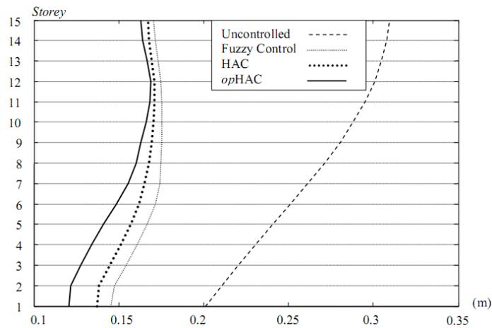
Figure 12. The maximum storey drift – Northridge earthquake
